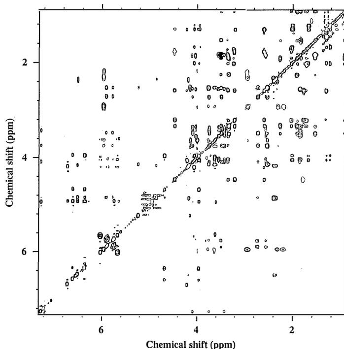
FIG. 3. HOHAHA spectrum of ciguatoxin-1 (CTX-1) at 500MHz in pyridine- $d_5$  (30°C). Chemical exchange between hydroxyl protons of CTX-1 and  $H_2O$  was detected as direct and relayed cross-peaks from each hydroxyl proton to the water resonance at 4.94ppm (mixing time 55msec). Data were zero filled to give a matrix consisting of 4 K x 1 K points.
