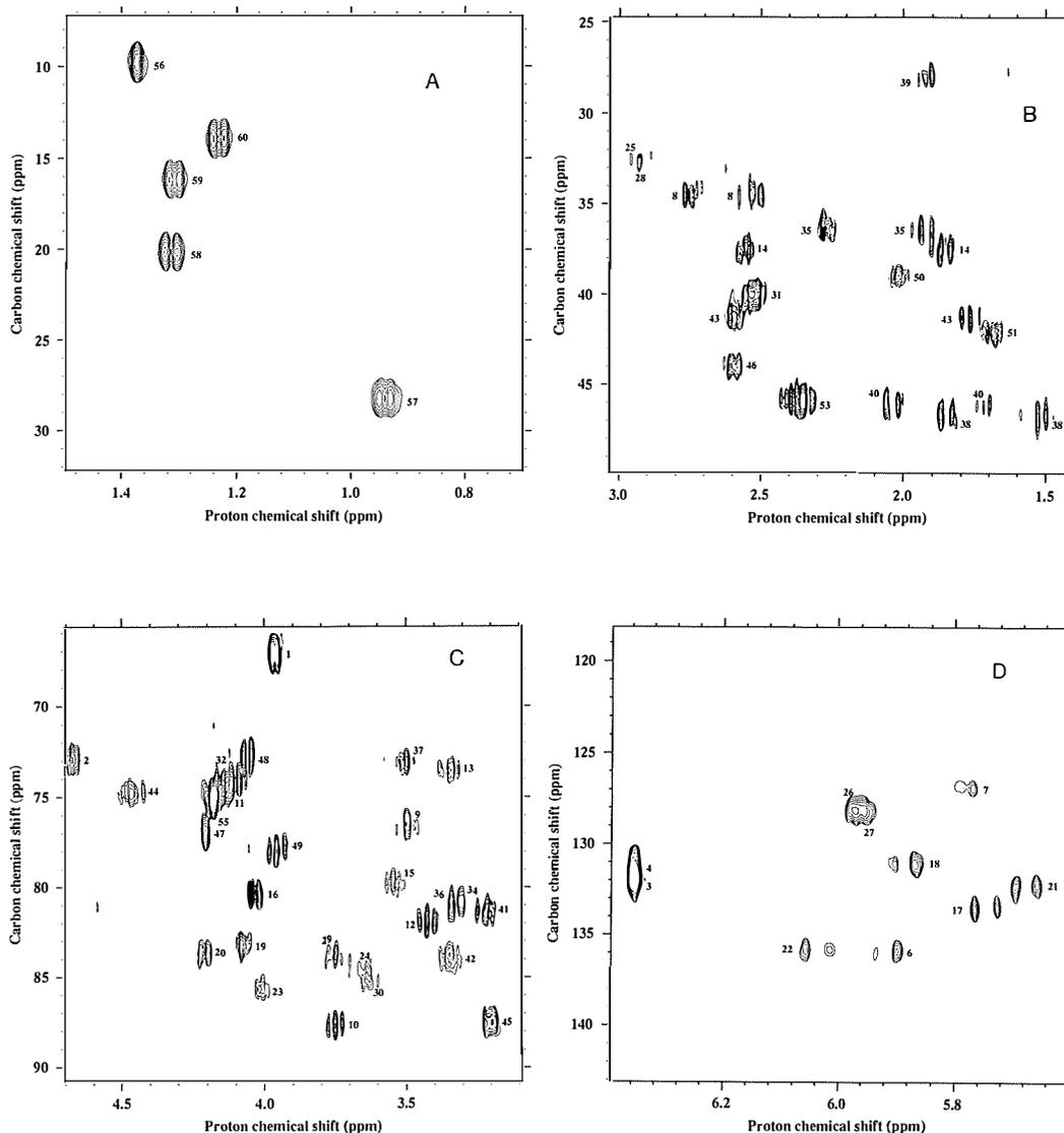
FIG.2. HMQC spectrum of ciguatoxin-1 (CTX-1) at 400 MHz in pyridine- $d_5$  (30°C).  $^1J_{CH}$  clustered into four regions shown in detail in panels A to D. Carbon number of the carbons giving rise to  $^1J_{CH}$  are labelled according to the structure of CTX-1 (Fig.1). Data were zero filled to give a matrix consisting of 4 K x 1 K points.
